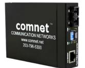
The ComNet CWFE2SC(M,S)2 Ethernet media converters are designed to transmit and receive 10/100 Mbps data over multimode or single mode optical fiber. The electrical interface will Auto-Negotiate to a 10 Mbps, or 100 Mbps Ethernet rate without any adjustments. The optical interface operates at a 100 Mbps Ethernet rate.
